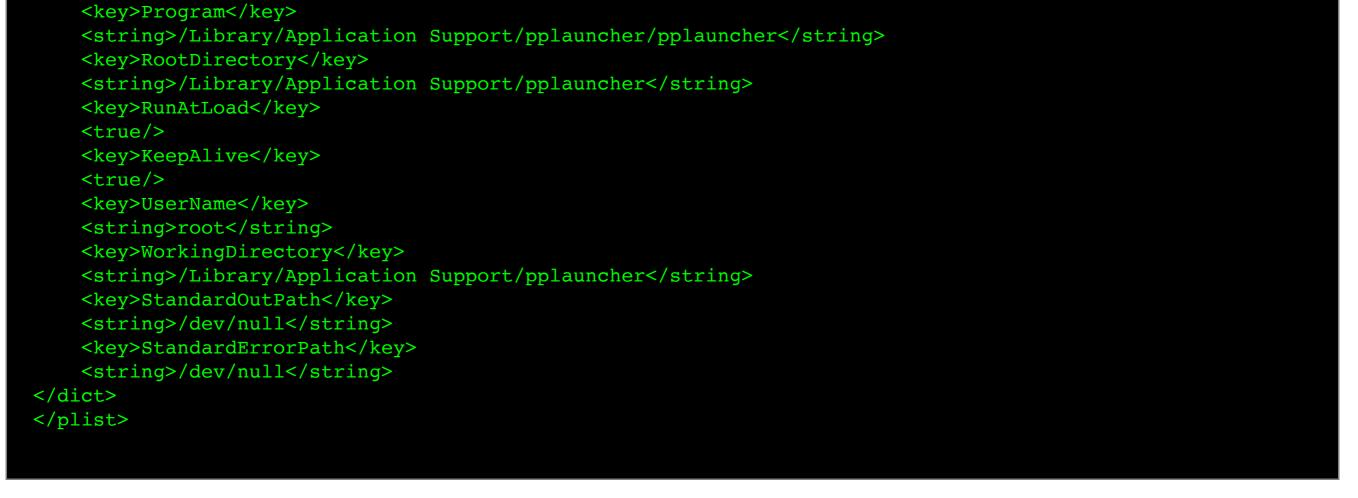
As the RunAtLoad key is the plist is set to true, pplauncher will be automatically (re)started each time the infected system is rebooted.
